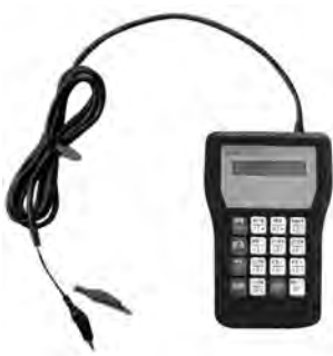
GSD-11K (Common Model Microcomputer Gas Meter / Communication Controller Setting Equipment)
